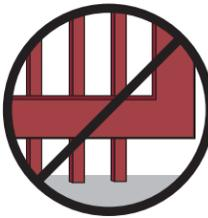
Gate MUST have a smooth bottom edge, no protrusions should exist.
